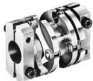
Fig. 24 A special purpose Huco-Pol double universal joint and drive gear supplied as a matched pair for a postal franking machine application. The generous offset capacity of the joint allows envelopes of varying thickness to be passed between the rubber impression rollers which are mounted on sprung radius arms.
